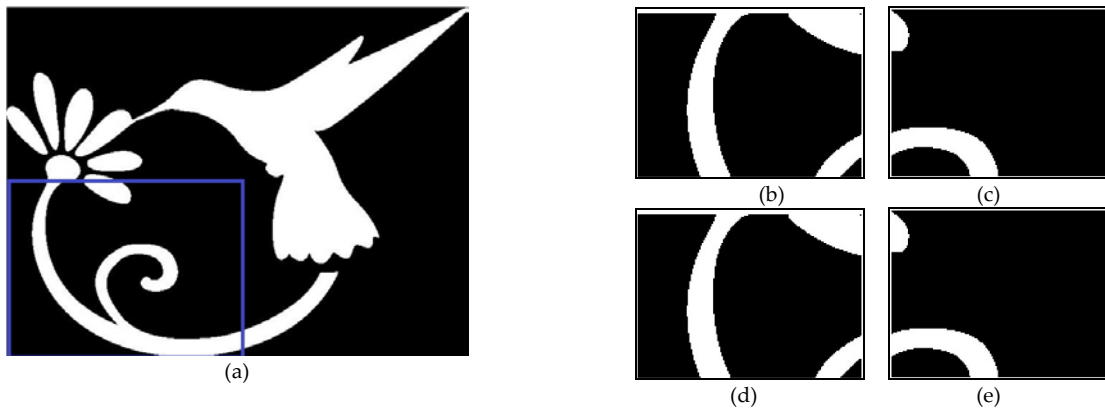
FIG. 5 THE PROCESS OF DIVIDING THE PICTURE INTO SEVERAL PARTS FOR SEARCHING THE BEST JUMP POINTS; (A) THE ORIGINAL PICTURE, (B) THE PART INCLUDE TWO OBJECTS, (C) THE PART INCLUDE TWO OBJECTS, (D) THE PART ONLY HAS ONE OBJECT, (E) THE PART ONLY HAS ONE OBJECT
